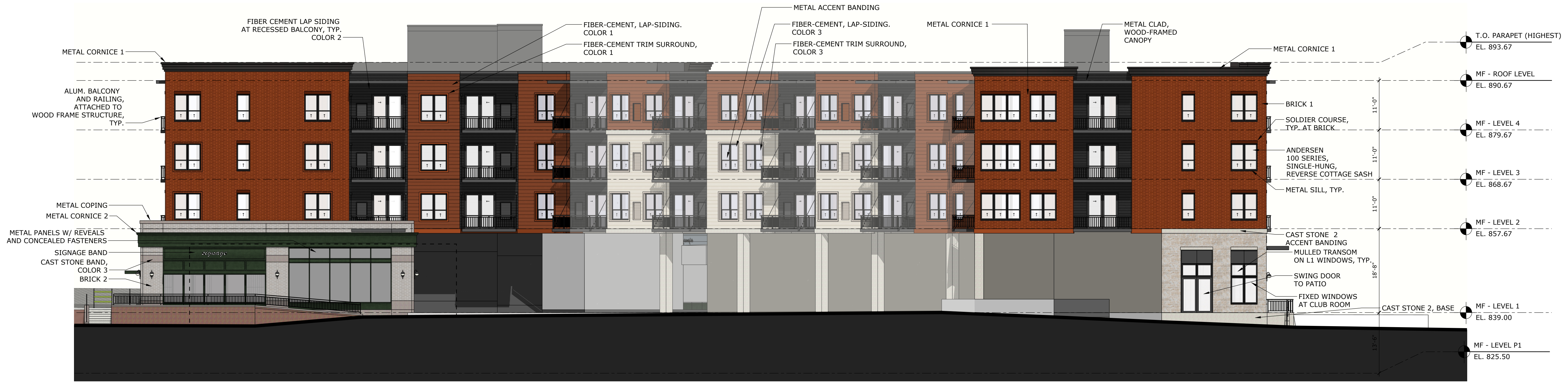
1 WEST ELEVATION SCALE: 3/32" = 1'0"
